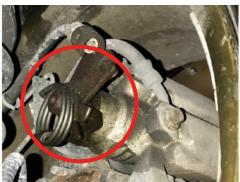
**Leaking, at the lever arm**Brake fluid is leaking around the lever arm.
